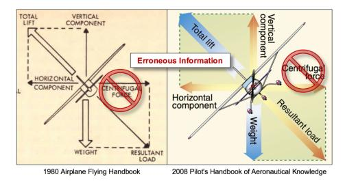
To answer the obligatory question "what turns an airplane," pilots memorize "the horizontal component of lift." That is an acceptable answer provided you are talking only about level turns, but airplanes are capable of climbing and descending turns, too. In the broadest sense, turns can occur in the horizontal, oblique, or vertical planes, and they occur for one simple reason: excess Lift (or alternatively, excess G).<sup>26</sup>
