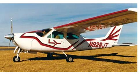
>>> Flying the Cardinal meant dealing with retractable gear and a variable pitch prop.
