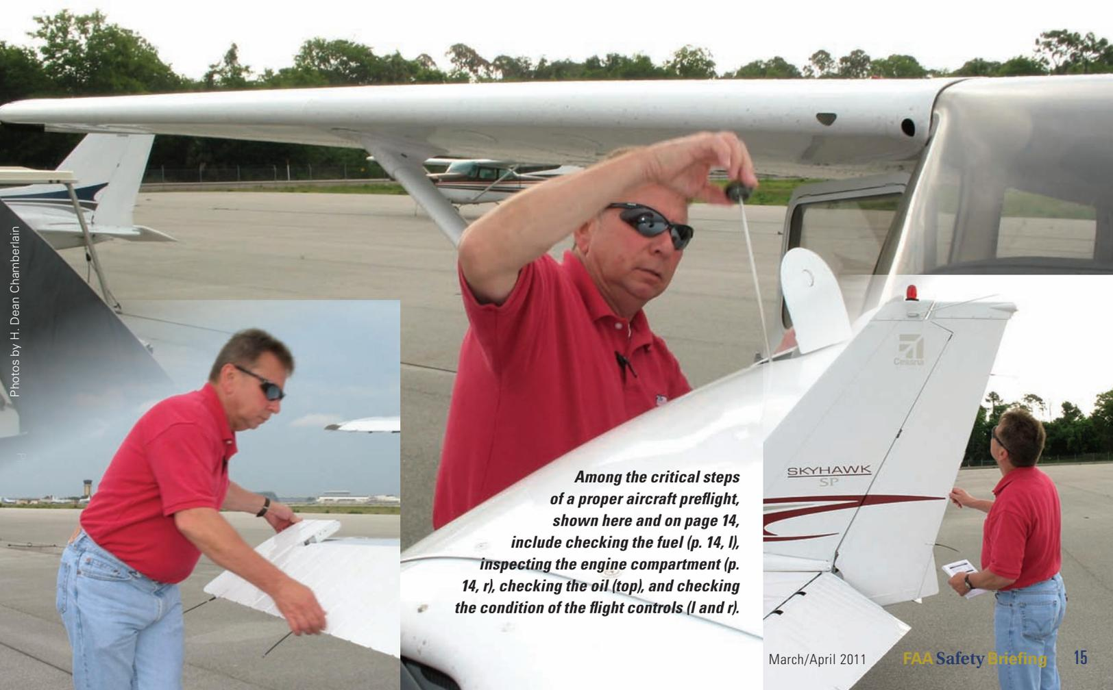
**Among the critical steps of a proper aircraft preflight, shown here and on page 14, include checking the fuel (p. 14, l), inspecting the engine compartment (p. 14, r), checking the oil (top), and checking the condition of the flight controls (l and r).**
