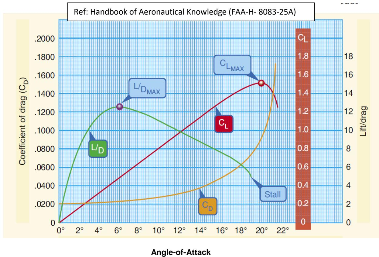
Figure 4:  $C_L$ ,  $C_D$ , and L/D ratio as a function of angle-of-attack
