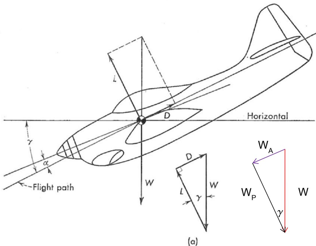
Figure 2: Force on the Aircraft in a Glide
