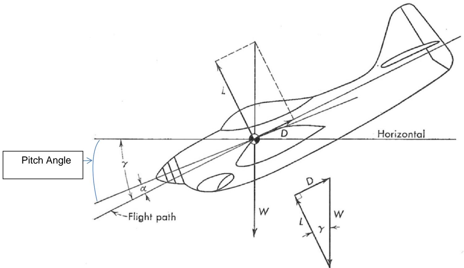
Figure 1: Forces on Aircraft in a Glide
